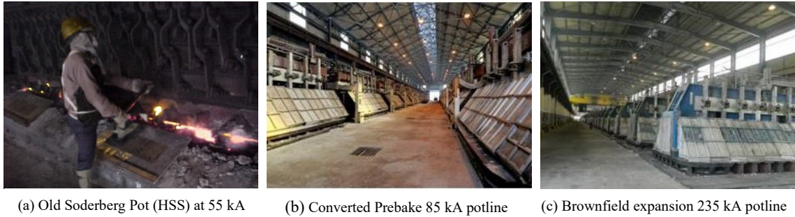
Figure 8. Hiralud smelter plant conversion and brownfield expansion.
